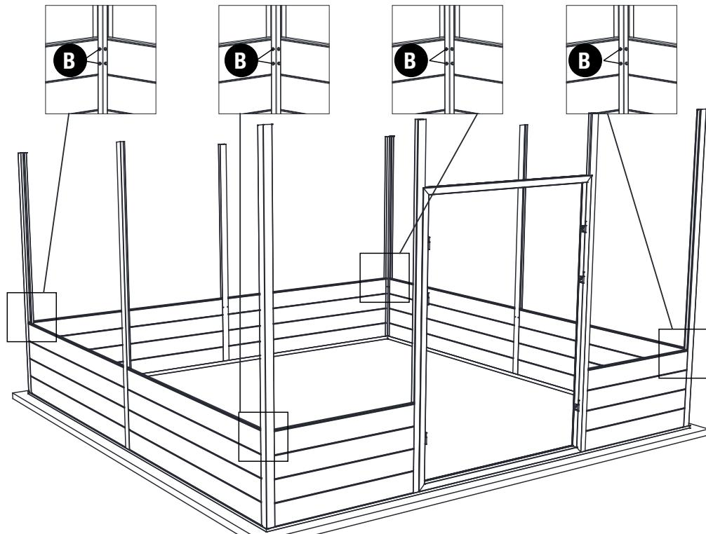
**EN** Install four rows of boards on all sides. Verify that the corner posts are plumb and then secure the assembly by placing two screws through the posts and into the wall boards. Repeat this procedure every fourth row.
