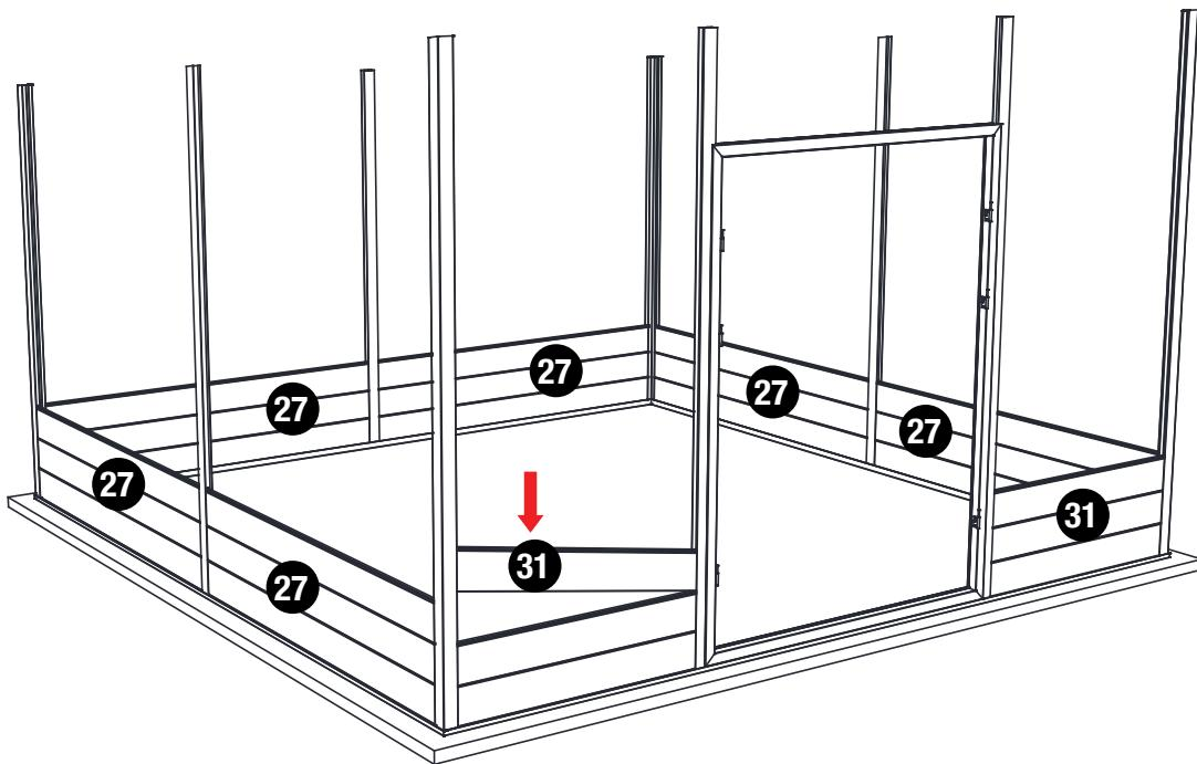
**EN** Apply a bead of clear silicone sealant into all posts channels and alternately slide wall panels into position.
