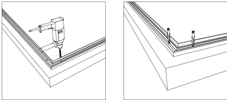
**EN** Install the eight posts with screws and corner angles. Verify that the posts are plumb and square to the sill plates before fixing them in position.
