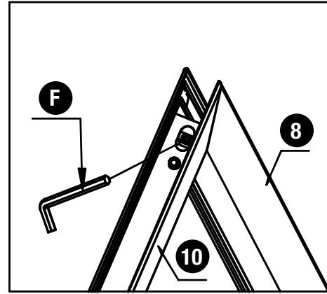
**EN** Assemble the door frame elements together as depicted by the drawings. Apply a bead of clear silicone sealant in all four door frame component channels. Slide the assembly in place.
