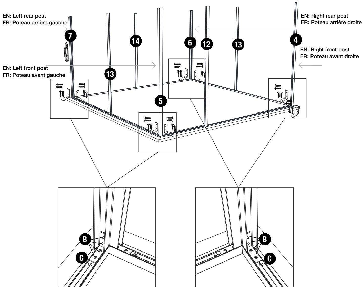
**EN** Install the eight posts with screws and corner angles. Verify that the posts are plumb and square to the sill plates before fixing them in position.
