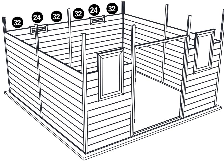
**EN** Install the vent traps after the 10th row of wall panels are in place. Fit the short wall panels as depicted in the drawing.
