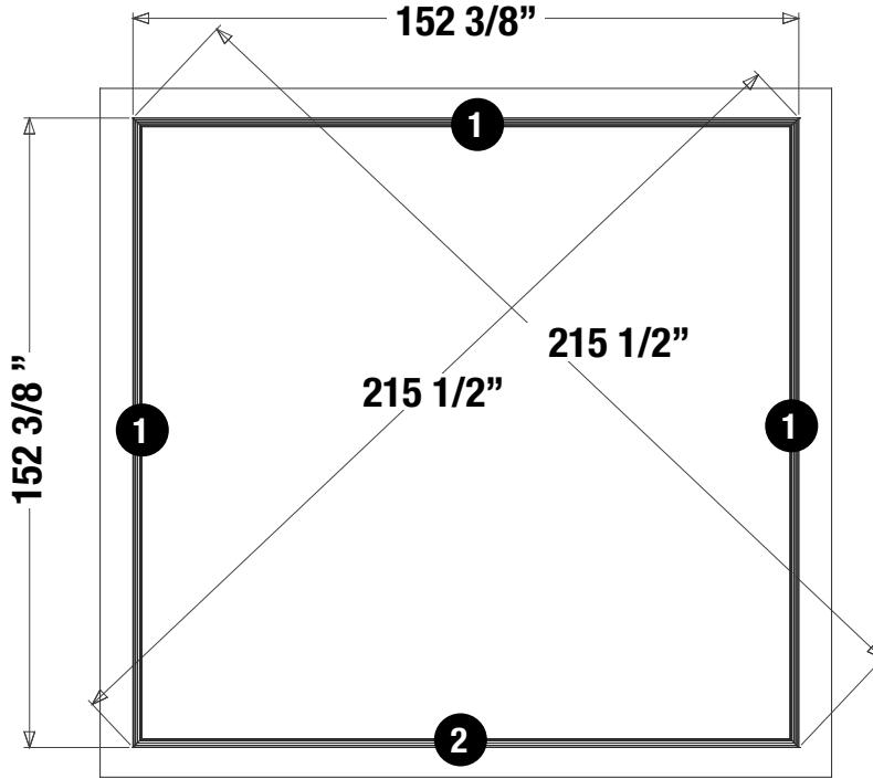
**EN** Layout and install the sill plates according to the dimensions provided with the drawings. Once this is done and that level has been checked, secure the sill plates with the proper fasteners.
