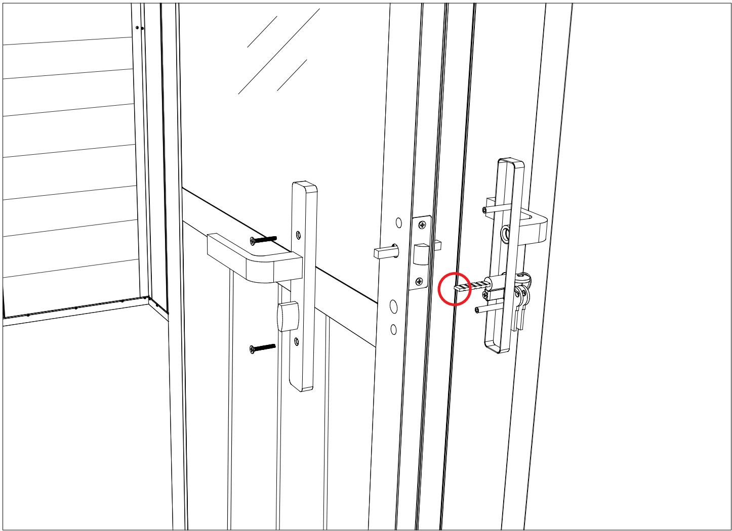
**EN** Cut the first section of the bar, then install the door handle assembly.
