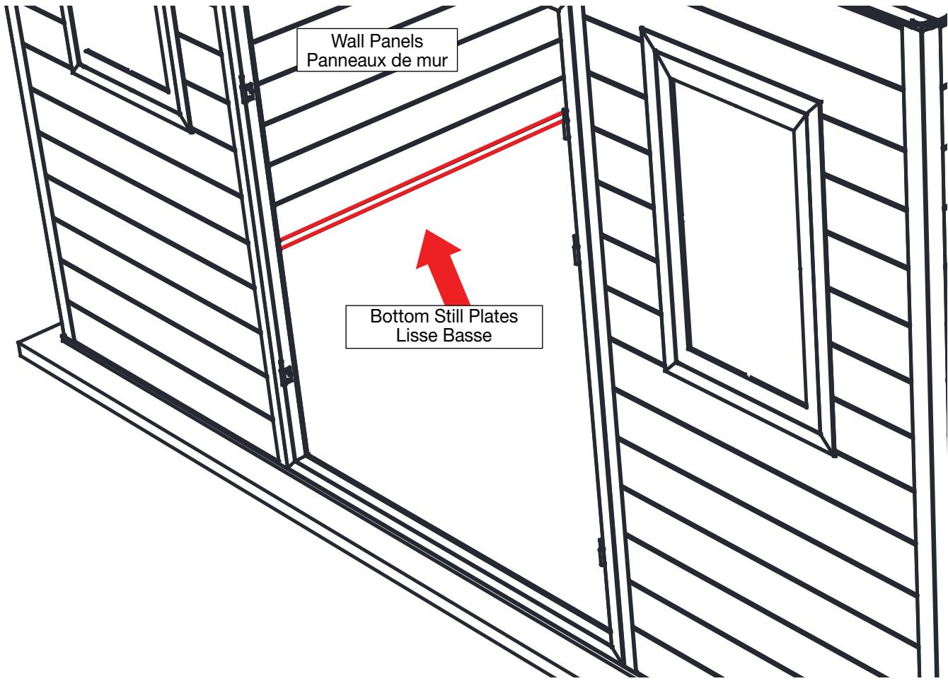
**EN** To prevent water infiltration, you must add a clear transparent bead of silicone at the bottom of the shed walls:
