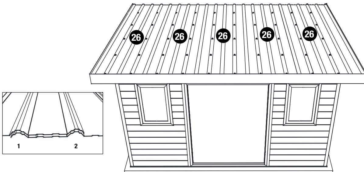
**EN** One by one, install the other panels. Subsequent roof panels must always overlap two ribs of the previous panel. Screw through both panels where they overlap. Do not screw into the fascias at this stage.
