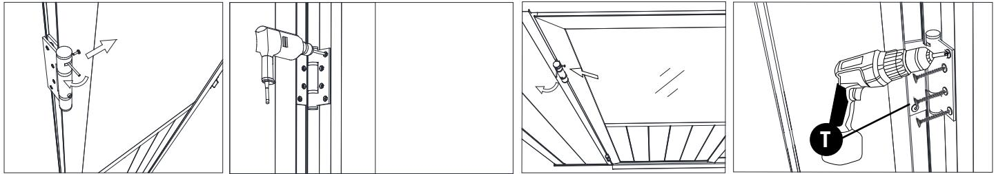
**EN** Insert the small peg into the regulating hole and push to the left in order to relieve the tension. Take out the locking pin from the hinge. Then position the door into the frame using shims and levers. Install the doors by fixing screws through the hinges and into the jambs. Re-tension the hinges springs to desired effect and insert back the locking pin. Cut the first section of the bar, then install the door handle assembly. Install the door latches.
