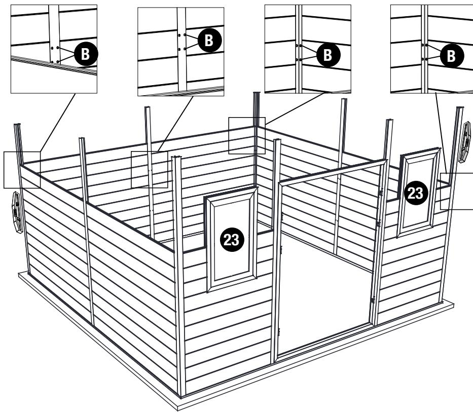
**EN** Verify that the corner posts are plumb and then secure the assembly by placing two screws through the posts and into the wall boards. Repeat this procedure every fourth row. Install the window kits. The windows can be installed so that they open towards the inside or the outside.
