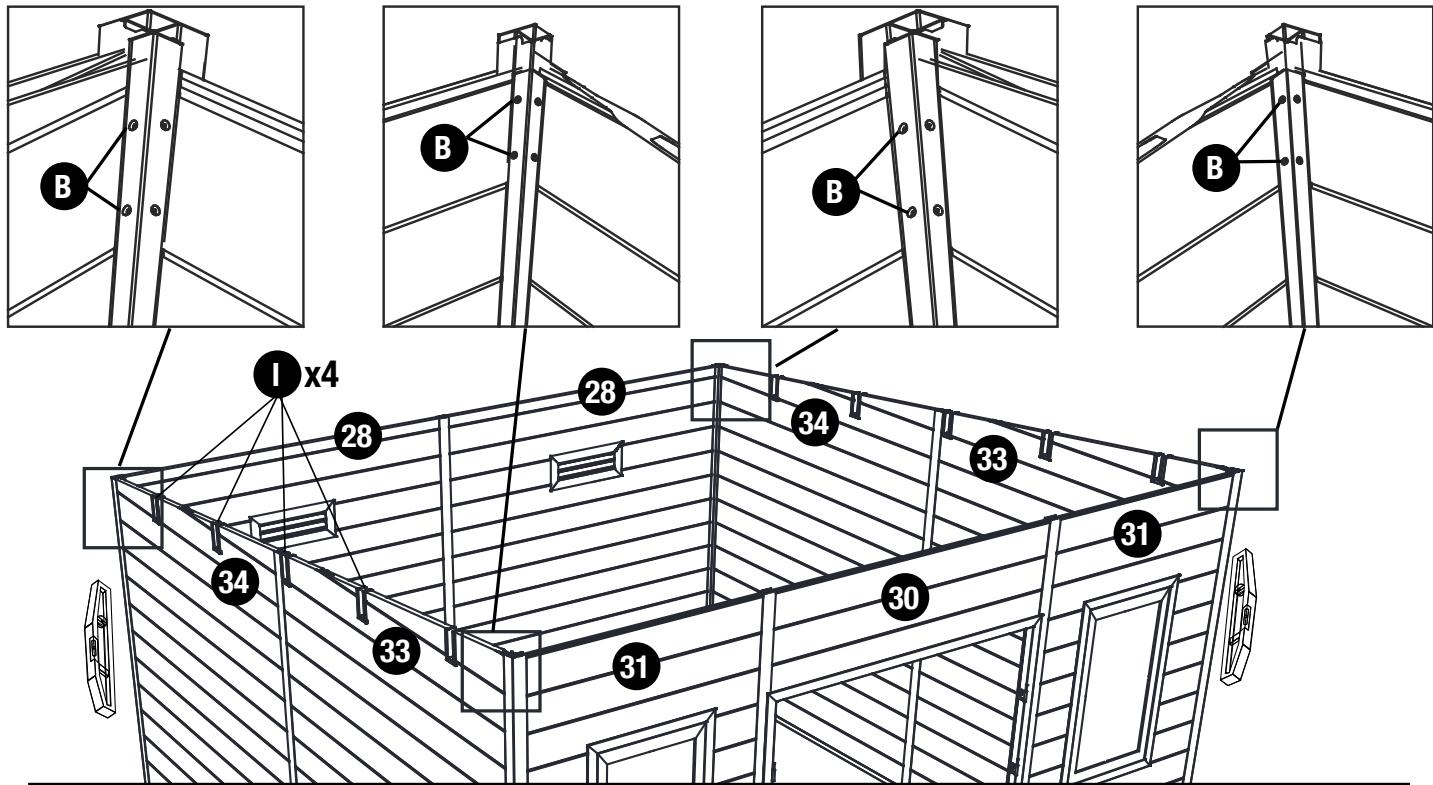
**EN** Install the gable wall assemblies. Secure them in place by putting two screws through the posts and into the wall boards at both ends. Slide the purlin gaskets in place
