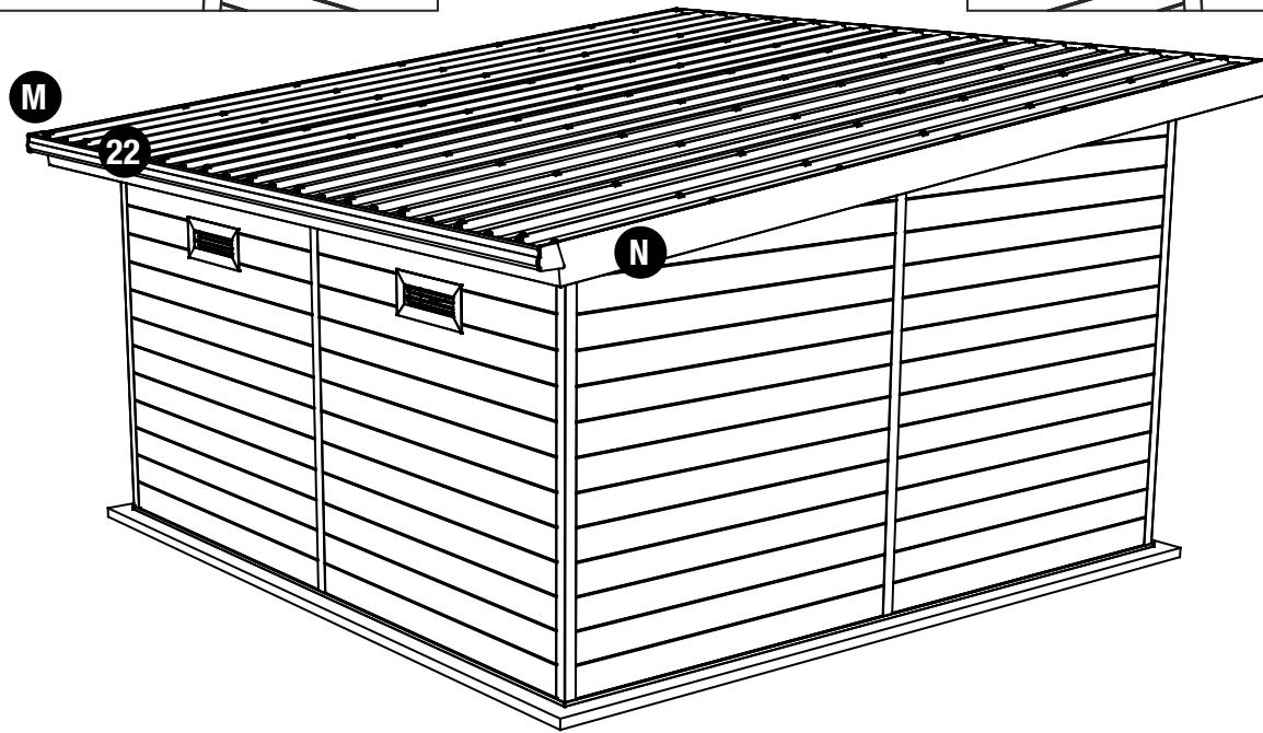
**EN** Slide the gutter's tab between the roof panels and the back fascia. Place a screw through a plastic screw cap, on every rib of the roof panels, into the fascia. Apply a bead of clear silicone sealant into the gutters' end caps' grooves and press in place. Now you can screw the roof panels into the perimeter.
