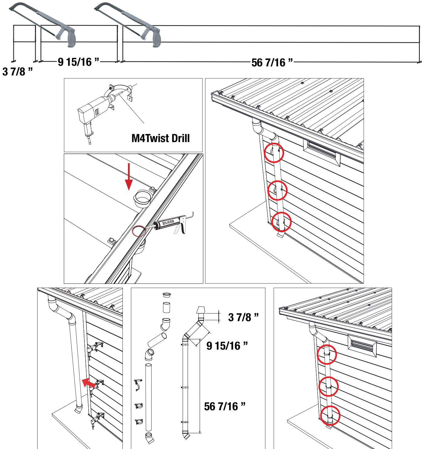
**EN** Cut the drain pipe into 3 pieces to the lengths shown above. We recommend to dry fit the downspout assembly into place and marking the desired pipe clamp locations before fixing them in place. Next, remove the assembly and screw the pipe clamps to the wall. Apply a bead of clear silicone sealant where the downspout connector will be in contact with the roof gutter. Replace the downspout and elbows and fix in place.
