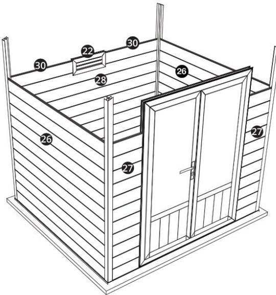
**EN** Install the vent traps after the 10th row of wall panels are in place. Fit the short wall panels as depicted in the drawing.
