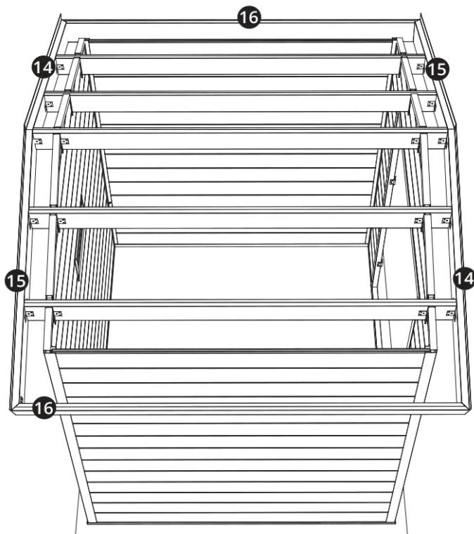
**EN** Insert and screw into the side fascias the Roof Brackets and Corner Angles. Install the fascias.
