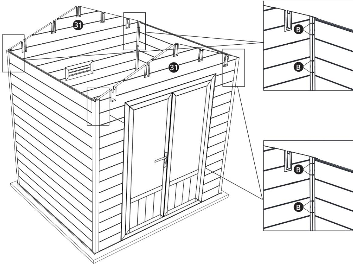
**EN** Install the gable wall assemblies. Secure them in place by putting two screws through the posts and into the wall boards at both ends. Slide the purlin gaskets in place.
