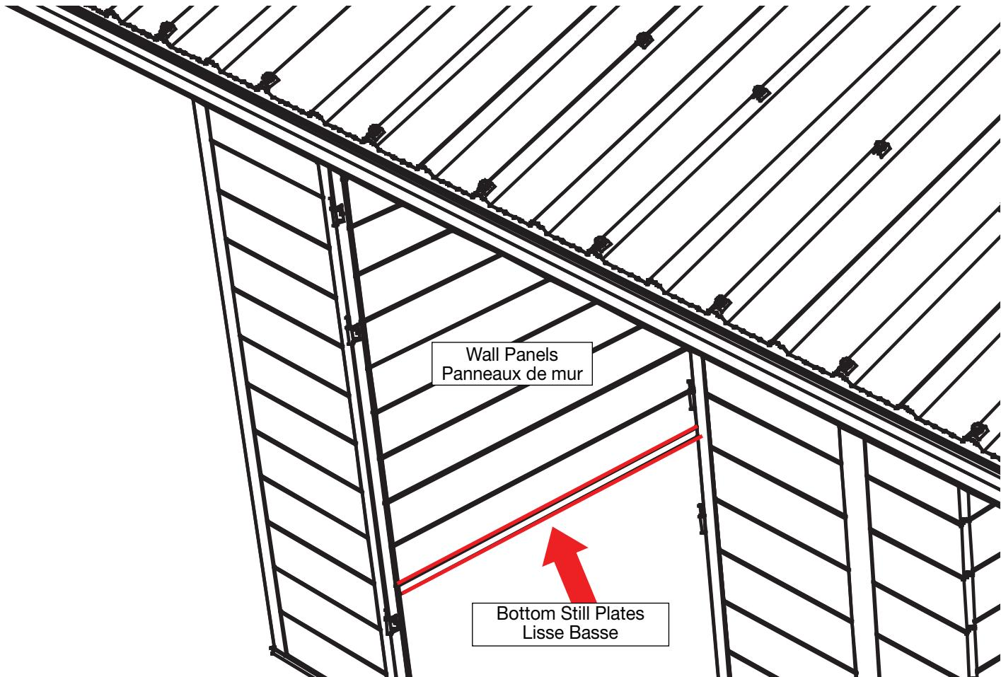
**EN** To prevent water infiltration, you must add a clear transparent bead of silicone at the bottom of the shed walls:
