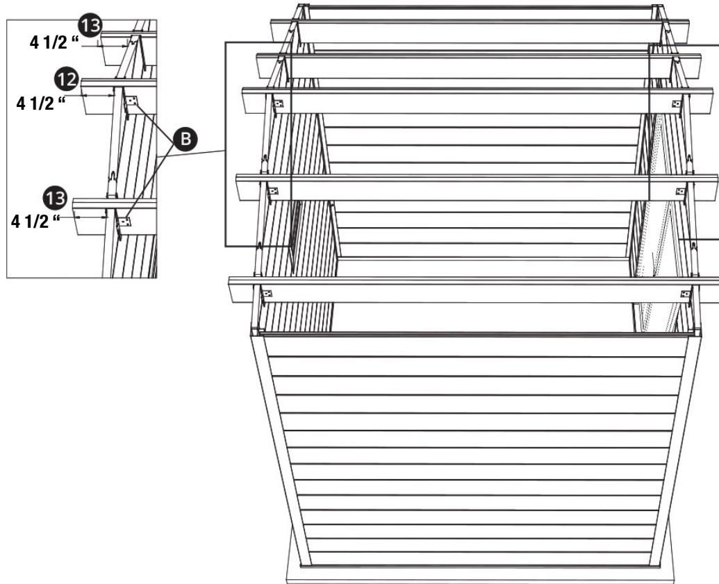
**EN** Install the corner angles to the ends of the purlins. Position the purlins into the slots so that they overhang the walls by 4 1/2 ". Secure them in place with screws and corner angles.
