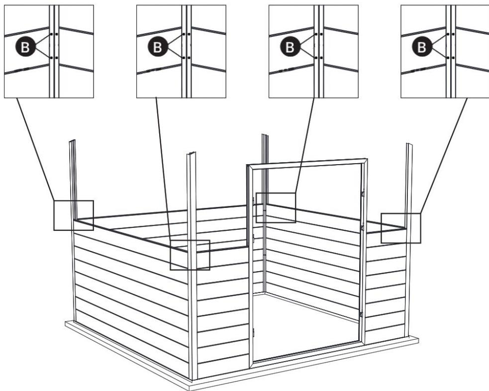
**EN** Verify that the corner posts are plumb and then secure the assembly by placing two screws through the posts and into the wall boards. Repeat this procedure every fourth row.
