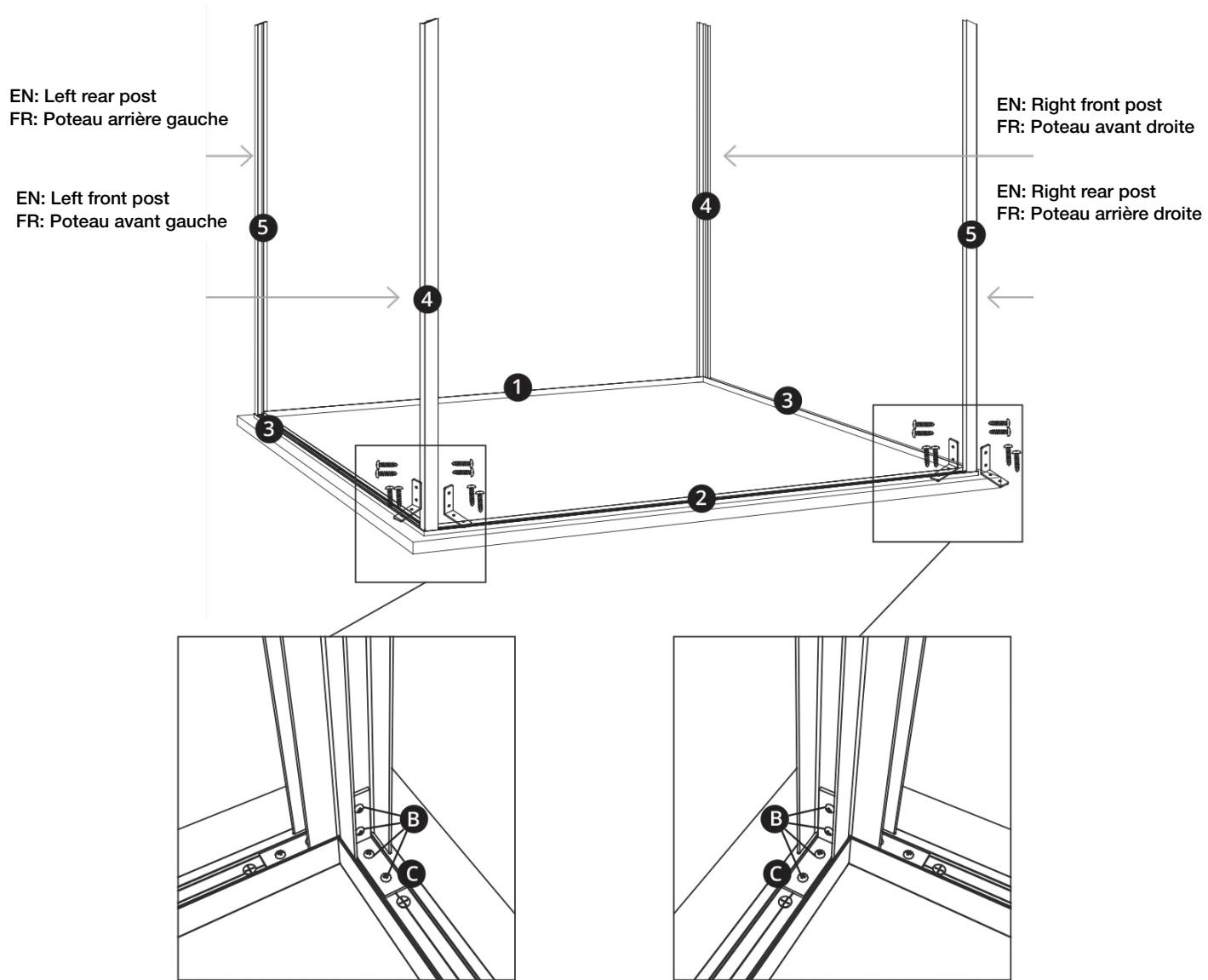
**EN** Install the four posts with screws and corner angles. Verify that the posts are plumb and square to the sill plates before fixing them in position.
