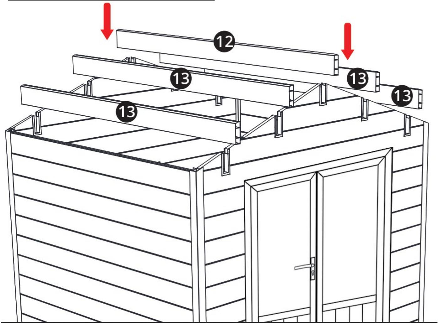
**EN** Install the corner angles to the ends of the purlins. Position the purlins into the slots so that they overhang the walls by 4 1/2". Secure them in place with screws and corner angles.
