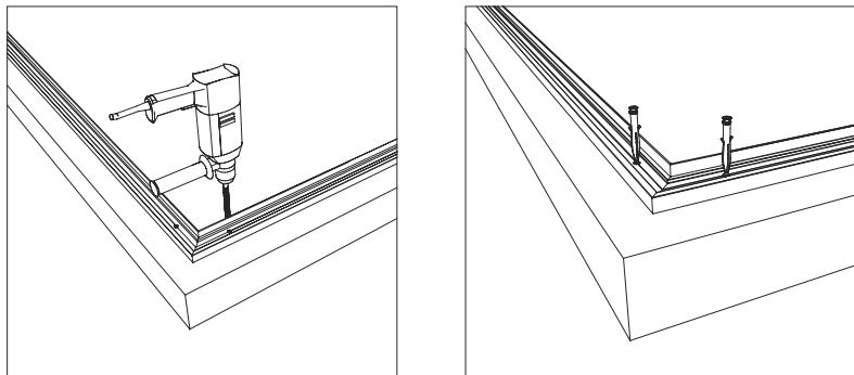
**EN** Layout and install the sill plates according to the dimensions provided with the drawings. Once this is done and that level has been checked, secure the sill plates with the proper fasteners.
